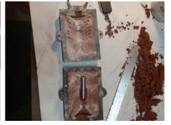
Finish prepping as before with the core inside the flask. The left picture shows the top of the core looking down the sprue. Cast your metal. The metal will flow around the
