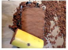
4) Scrape or skree excess sand off with the ruler so the sand is level with the top of the flask. Under or over filling will cause your mold to be unstable which will affect your casting.
