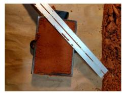
5) Coat the object to be cast in talc. The talc acts as parting powder allowing you to easily remove your object from the sand.
