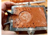
19) Re-assemble the cope and drag and make sure it is a snug fit. Clamps or a binder may be needed to make sure the halves do not come apart during casting.
