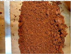
2) Fill drag with sand. Sifting sand into the drag is optional. Sifting breaks the sand up a little more. I have the same results whether I sift or not.
